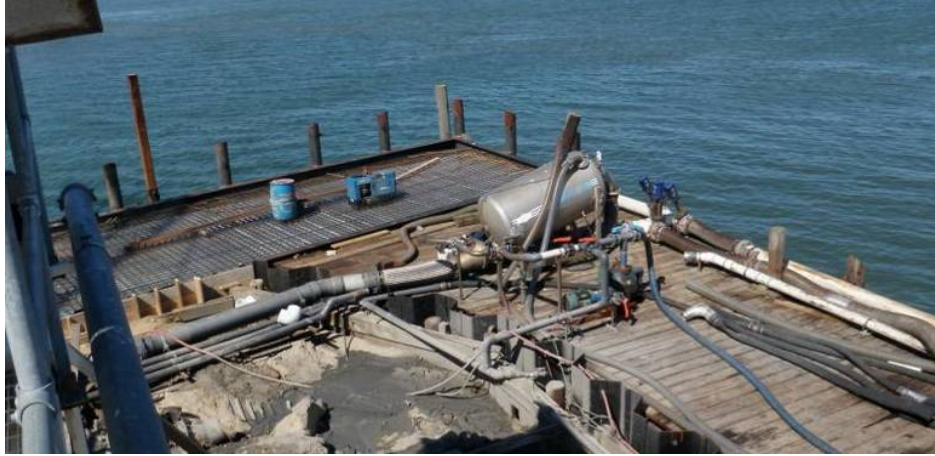
Figure 22. A dockside pump utilized for removing fish from the hold and into the processing facility.
