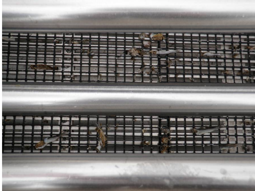
Figure 5. Detail of the lower half of a de-watering box, demonstrating how small marine life and detritus can catch and clog on the mesh
